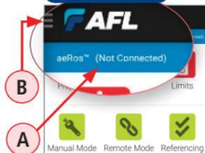
Once the TURBO™ app is launched on a smart device, the Home screen is the first screen you see on the application startup. If you haven't logged in to aeRos, notice that connection status **A** indicates 'Not Connected'.
